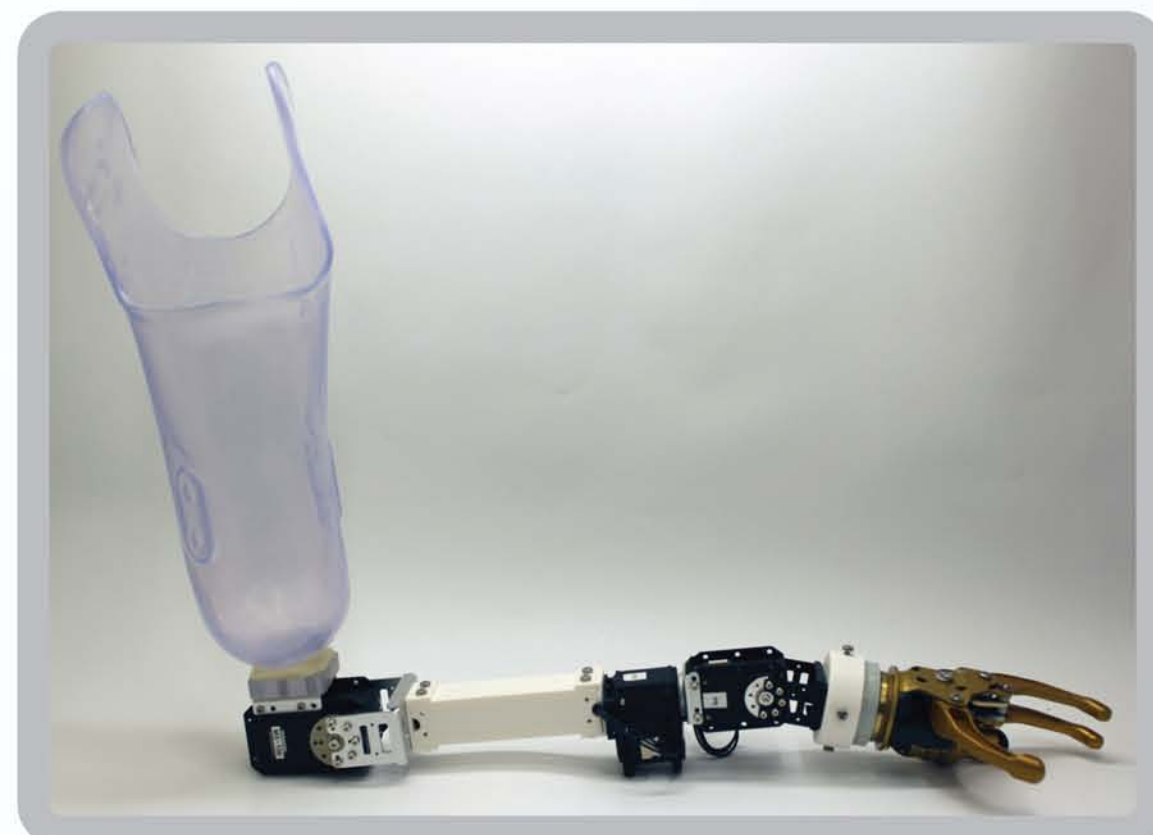
Adapter allows arm to be mounted to a prosthetic socket from the elbow down.
