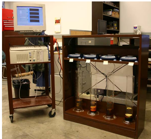
Figure 3.2 a) Horizontal and vertical imbibition tubes b) measurement using scales.
