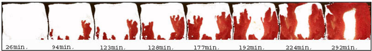
Figure 8.8 c-Experiment V1 (counter-current, mineral oil) 2D visualization experiment. (OOIP: Original Oil In Place)
