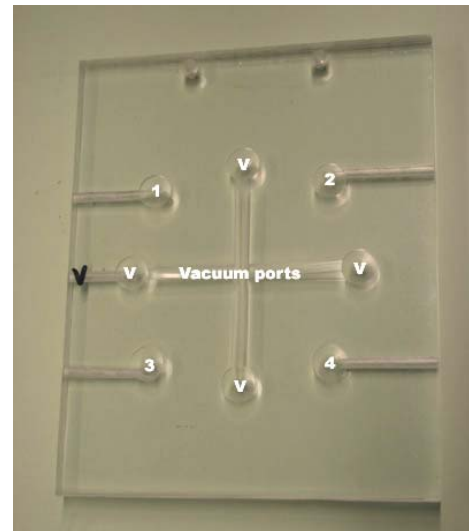
Figure 3.6 a) Glass model on holder, inlet-outlet ports connected, vacuum port disconnected. Ports on the model are marked with numbers. Ports 1&2 and 3&4 are connected with fracture which is highlighted with gray lines, b) model holder with four configurable ports and one vacuum port. Vacuum suction cups are connected to vacuum port internally.
