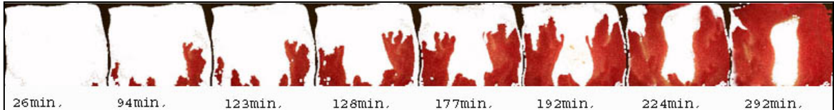
Figure 6.25 Experiment on 2-D glass bead model (white: mineral oil, red: solvent (pentane)).
